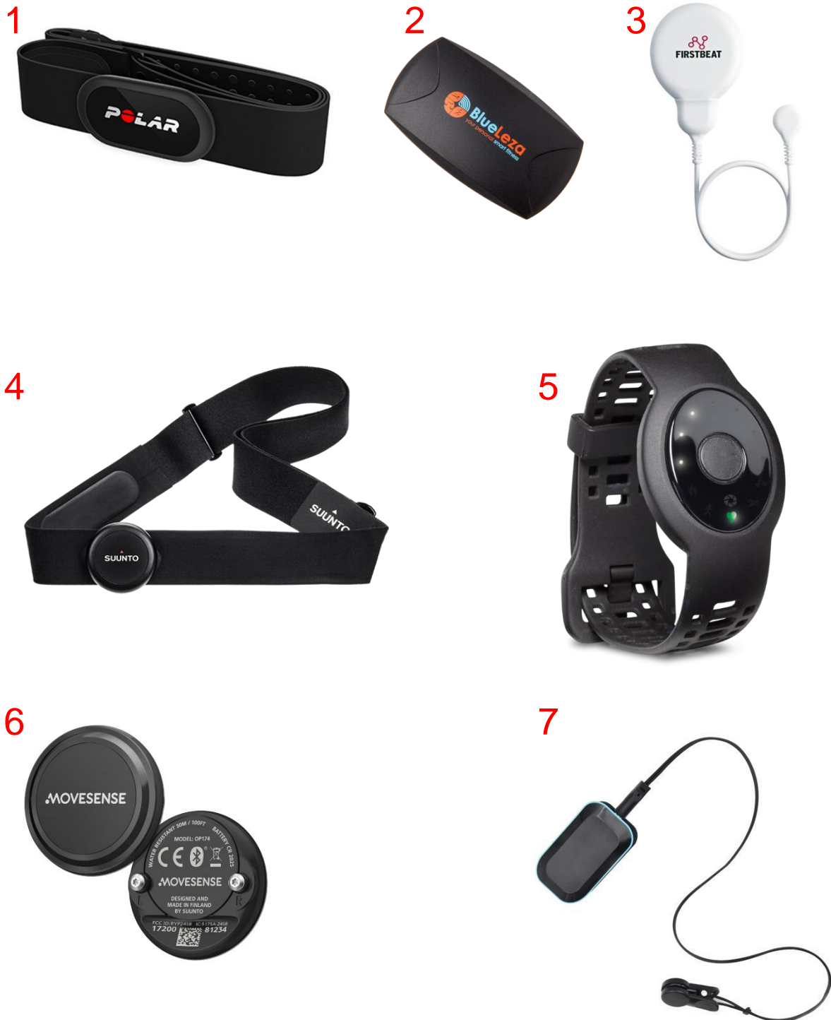
Figure 26: Images of the used biosensors at Subject Testing 1+2; 1=Polar H10 [53]; 2=HRM Blue [54]; 3=Firstbeat Bodyguard [55]; 4=Suunto Smart Sensor [56]; 5=Zoom HRV [57]; 6=Movesense HR [58]; 7=HRM-2935 [59]
